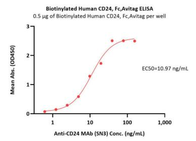
Immobilized Biotinylated Human CD24, Fc,Avitag (Cat. No. CD4-H82F5) at 5  $\mu$ g/mL (100  $\mu$ L/well) on Streptavidin (Cat. No. STN-N5116) precoated (0.5  $\mu$ g/well) plate, can bind Anti-CD24 MAb (SN3) with a linear range of 0.6-20 ng/mL (QC tested).
