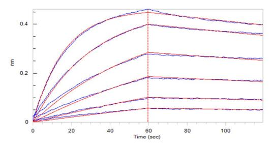
Loaded Biotinylated Mouse FcRn Heterodimer Protein, Avitag, His Tag&Twin-Strep Tag (Cat. No. FCM-M82W6) on SA Biosensor, can bind Herceptin with an affinity constant of 3.38 nM as determined in BLI assay (ForteBio Octet Red96e) (QC tested).
