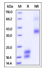
Biotinylated Human VEGF121, Avitag, His Tag on SDS-PAGE under reducing (R) and non-reducing (NR) conditions. The gel was stained with Coomassie Blue. The purity of the protein is greater than 95%.
